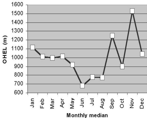
**Fig. 2 . Annual variation of Optimum Coupling heights for Elevated Ducts.**
