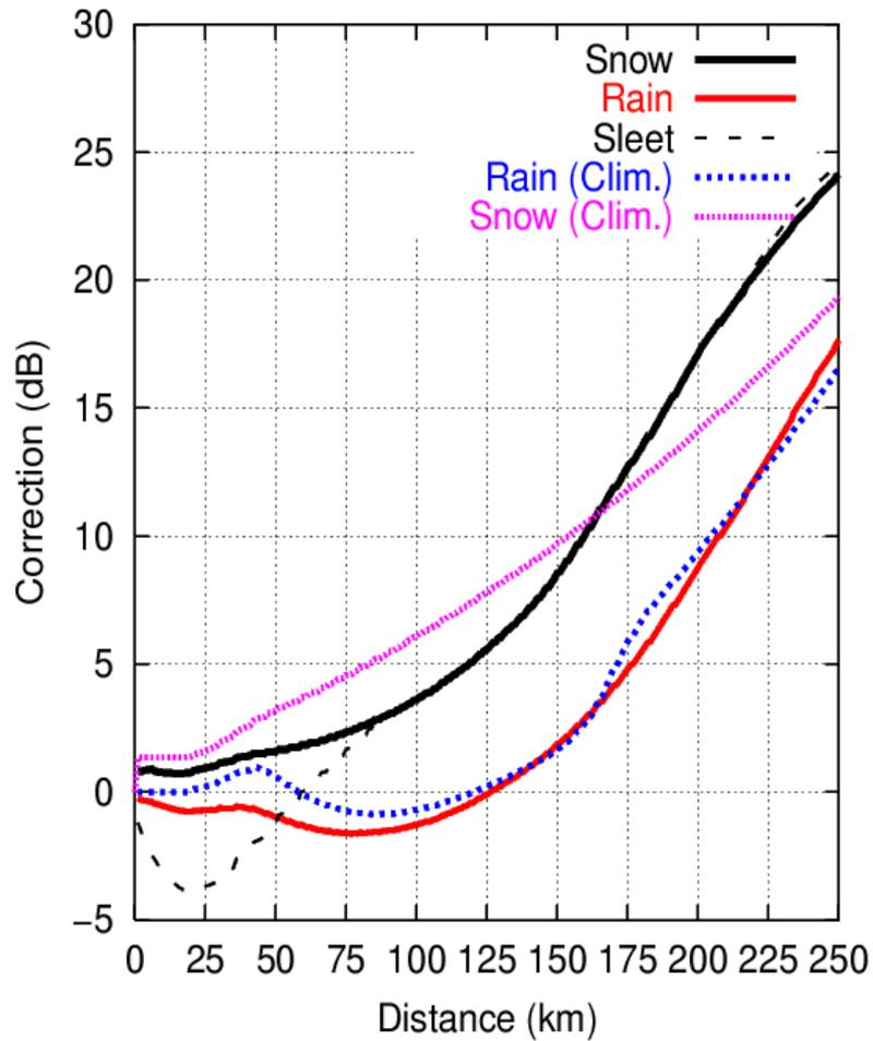
Fig. 7. – Yearly average VPR correction based on all measured profiles (Snow, Rain, Sleet) and on the climatological profiles (Clim.)
