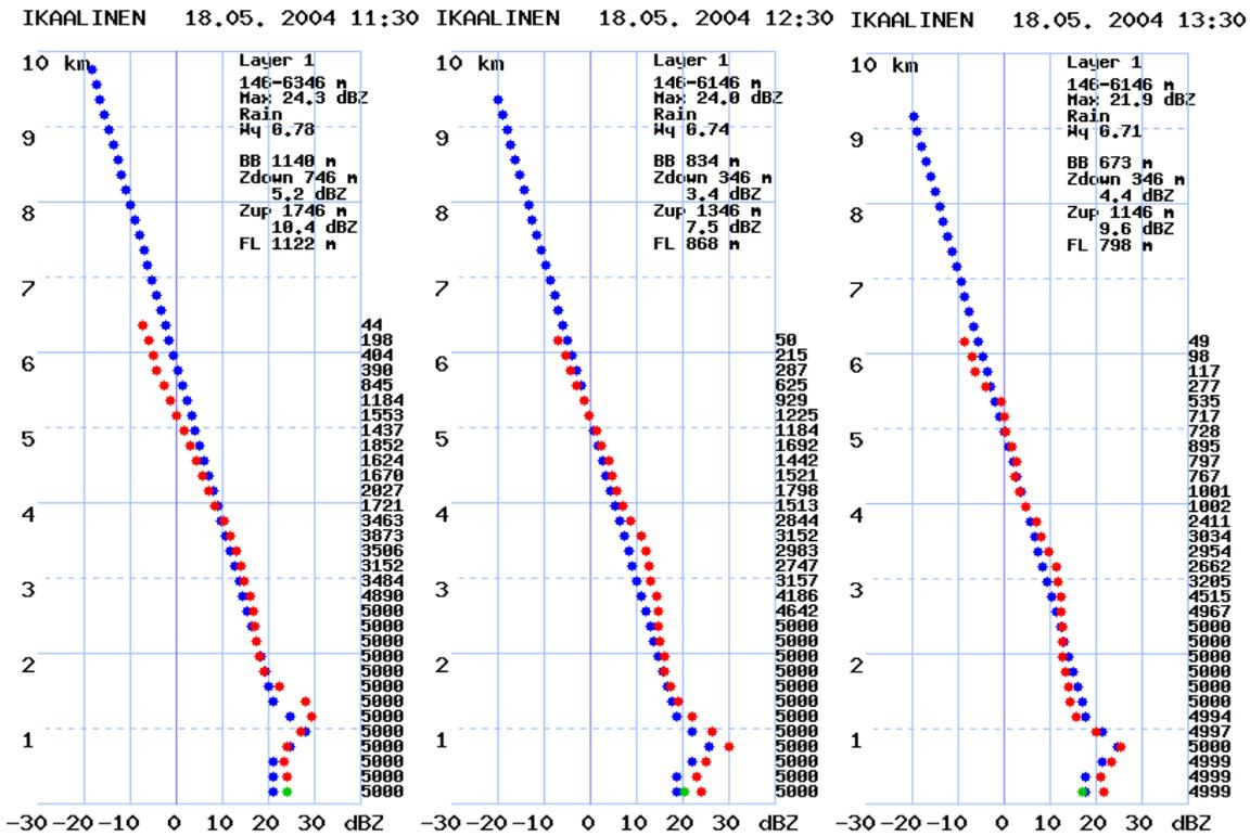
Fig. 8 – Measured VPR (red) and climatological VPR (blue) based on freezing level height from NWP model HIRLAM measured at Ikaalinen radar.
