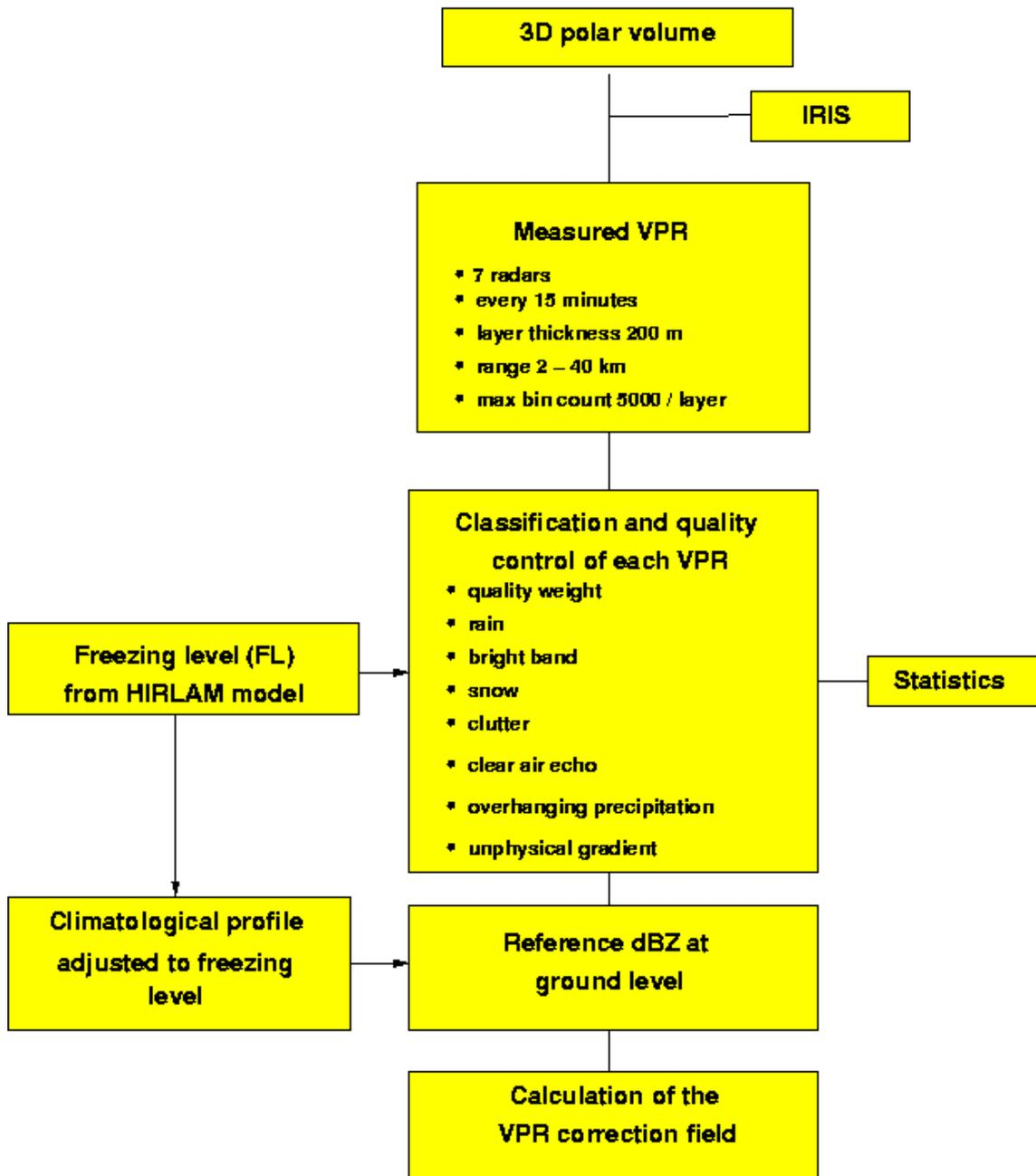
Fig. 5 – VPR correction steps in the radar network of Finnish Meteorological Institute.
