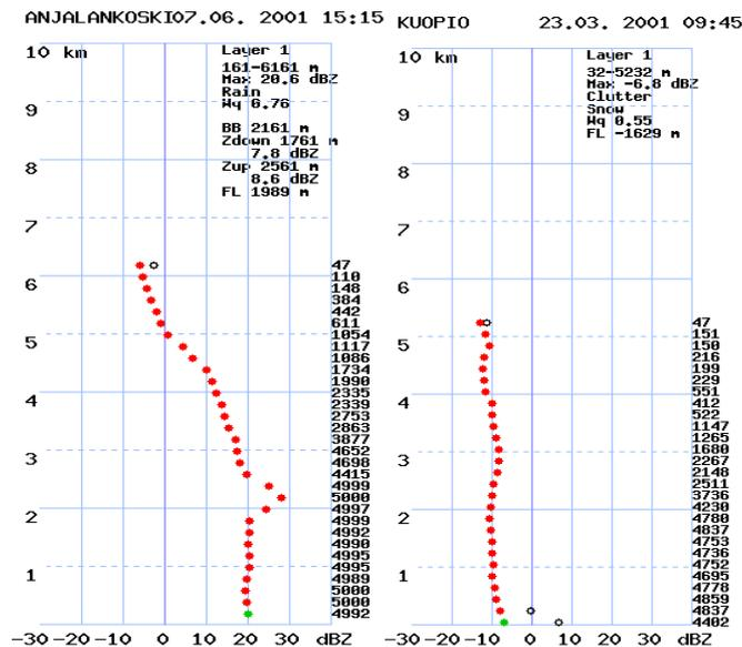
Fig. 1 – Typical rain profile with bright band and snow profile with clutter.
