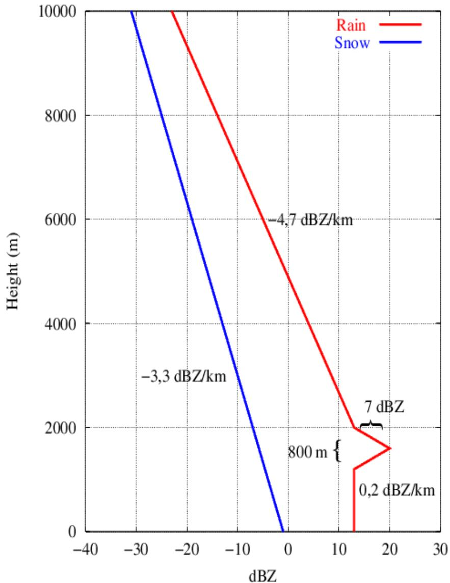
Fig. 4 – Climatological profiles for snow and rain based on precipitation profiles from March 2001 to August 2003. Note that only shape, not the actual dBZ values do effect on the magnitude of the VPR correction.
