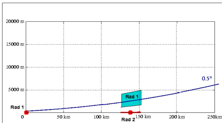
Fig. 11 – The validation method of the VPR correction based on radar pairs in the radar network of FMI.
