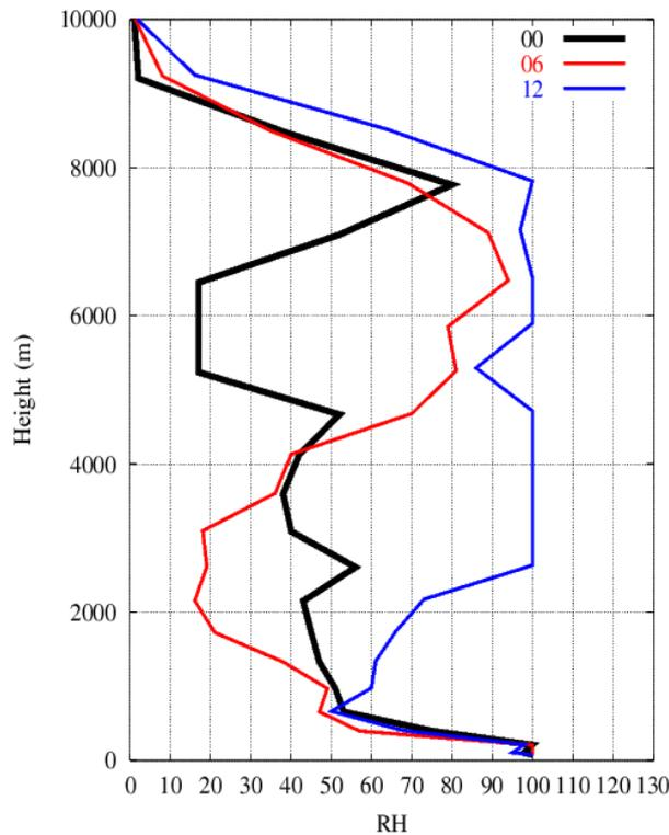
Fig. 10 – An example of the vertical distribution of relative humidity obtained from the NWP model HIRLAM at the radar site Utajärvi during a period of OP.
