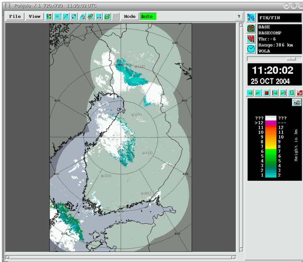
Fig. 2 – An example of precipitation base height field composite in Finnish radar network. All blue and green areas indicate that the height of the precipitation base is located above the ground
