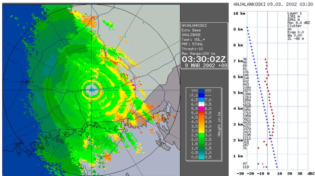
Fig. 1 – An example of the height overhanging precipitation (km) above Anjalankoski radar and classified VPR measured at the same time
