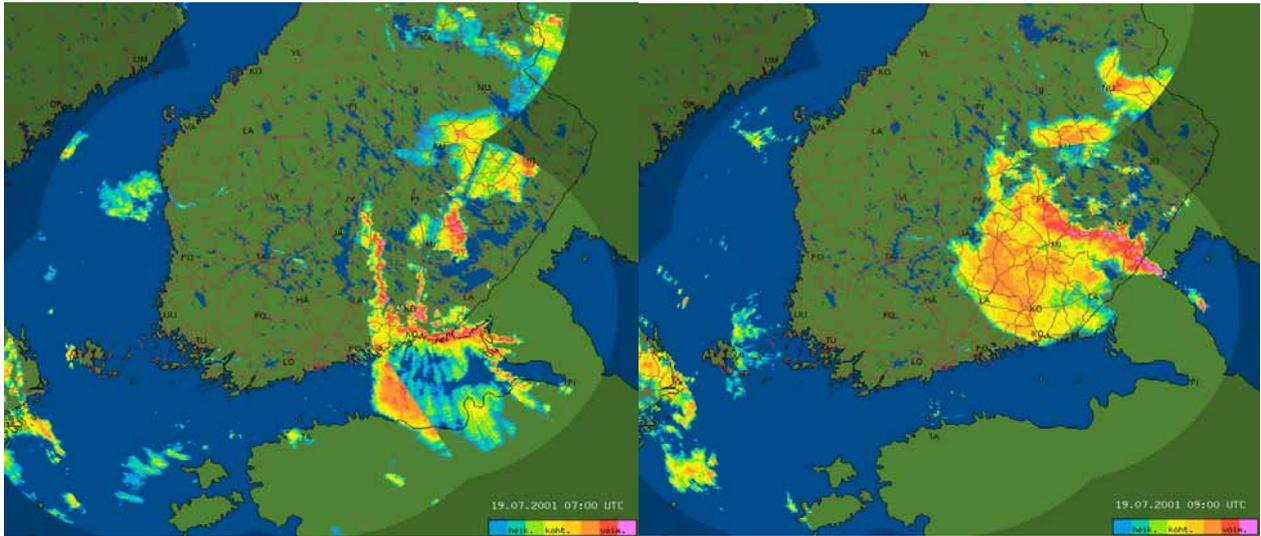
Fig. 4 – Severe attenuation case in summer time MSC. In the left panel can be seen strong attenuation south of strong convective cells causing seam in radar composite in that area. In the left panel MSC is north of Anjalankoski radar and radar beam is not anymore attenuated in that area.
