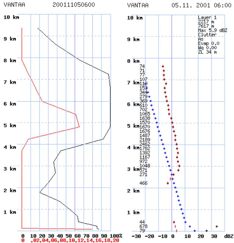
Fig. 3 – Measured VPR (right panel), specific cloud condensate (red) and relative humidity (black) (left panel) from the NWP model HIRLAM 6 hour forecast in an overhanging precipitation case.
