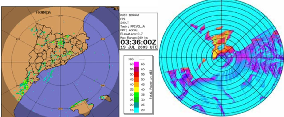
Fig. 8 – (a) observed radar image (b) Full simulation of the anomalous propagation echoes using data from the NWP model
