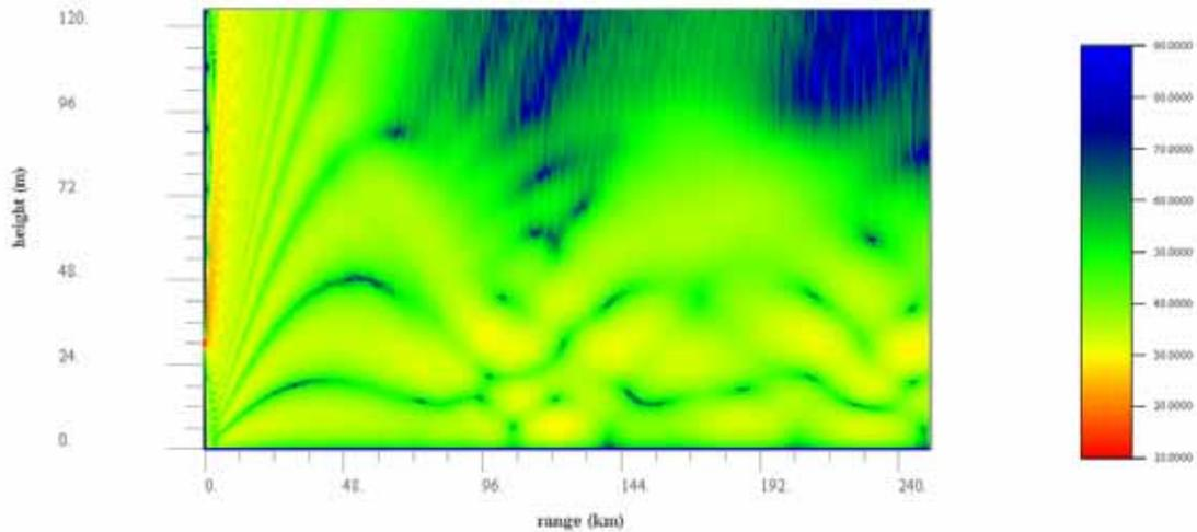
Fig. 7 – Tests of the PEM implementation over flat terrain (conformal with earth curvature). (a) above, in a normal atmosphere; fringes occur in the region of weak field outside the main beam, where energy reflected by the surface interferes with the free-space field. (b) below, with an elevated duct at 100 m; Energy at high angles is not trapped, but at low angles, the radiation pattern comprises a mixture of waveguide modes.
